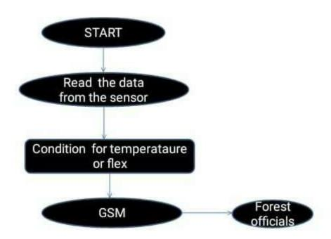
When the data readed from flex sensor, flame sensor, infrared sensor satisfy the given condition or threshold valve it will trigger the buzzer, and sends information to forest officials which provide an information such as tree name ,location and perfect location of tree. If forest fire occurs in forest it will send the information to forest officials.
