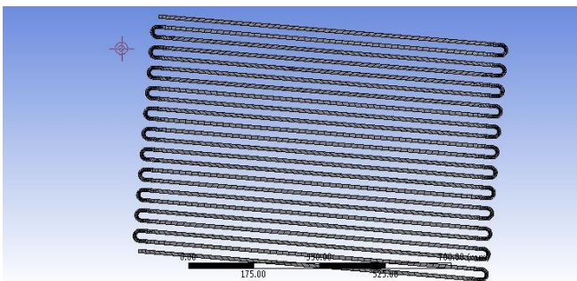
Fig – Meshed Model
