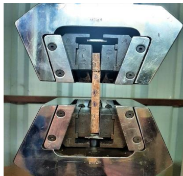
Fig: 8 Tensile testing on UTM.
