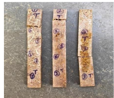
Fig: 9 Specimens after Tensile testing.
