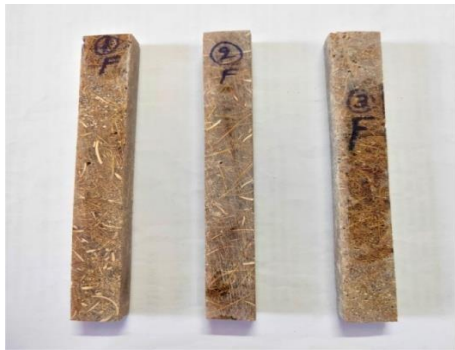
Fig: 15 Flexural test Specimens. Three point bending test for specimen. Specimens after Flexural test.
